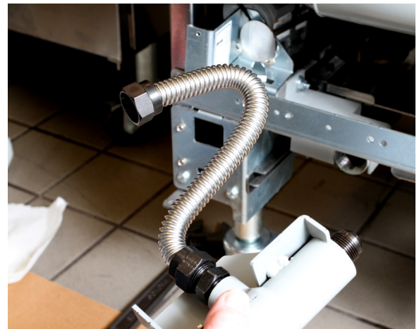
Figure 3 : Shape the flexline attached to the pre-filter to route to the filter pan pickup.
